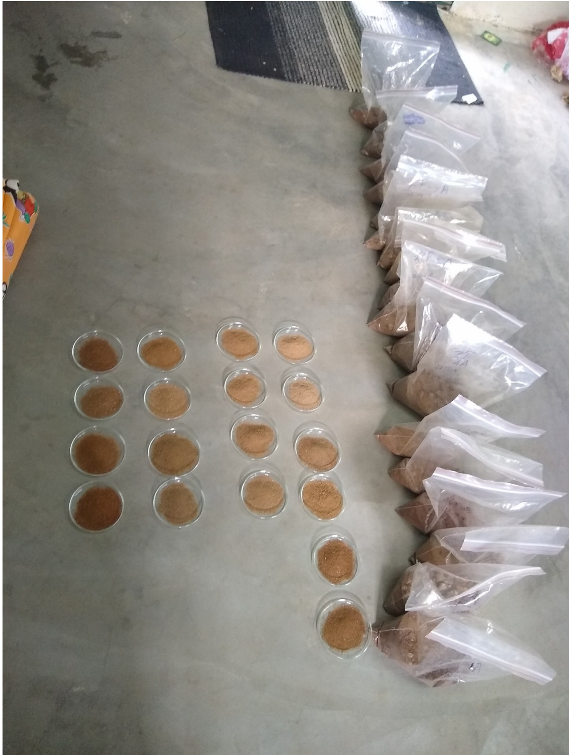
Figure 8: Soil samples and soil sub samples. From the soil samples collected, sub samples of 15-20 g were taken, weighed before and after drying in the hot air oven to calculate soil moisture.
