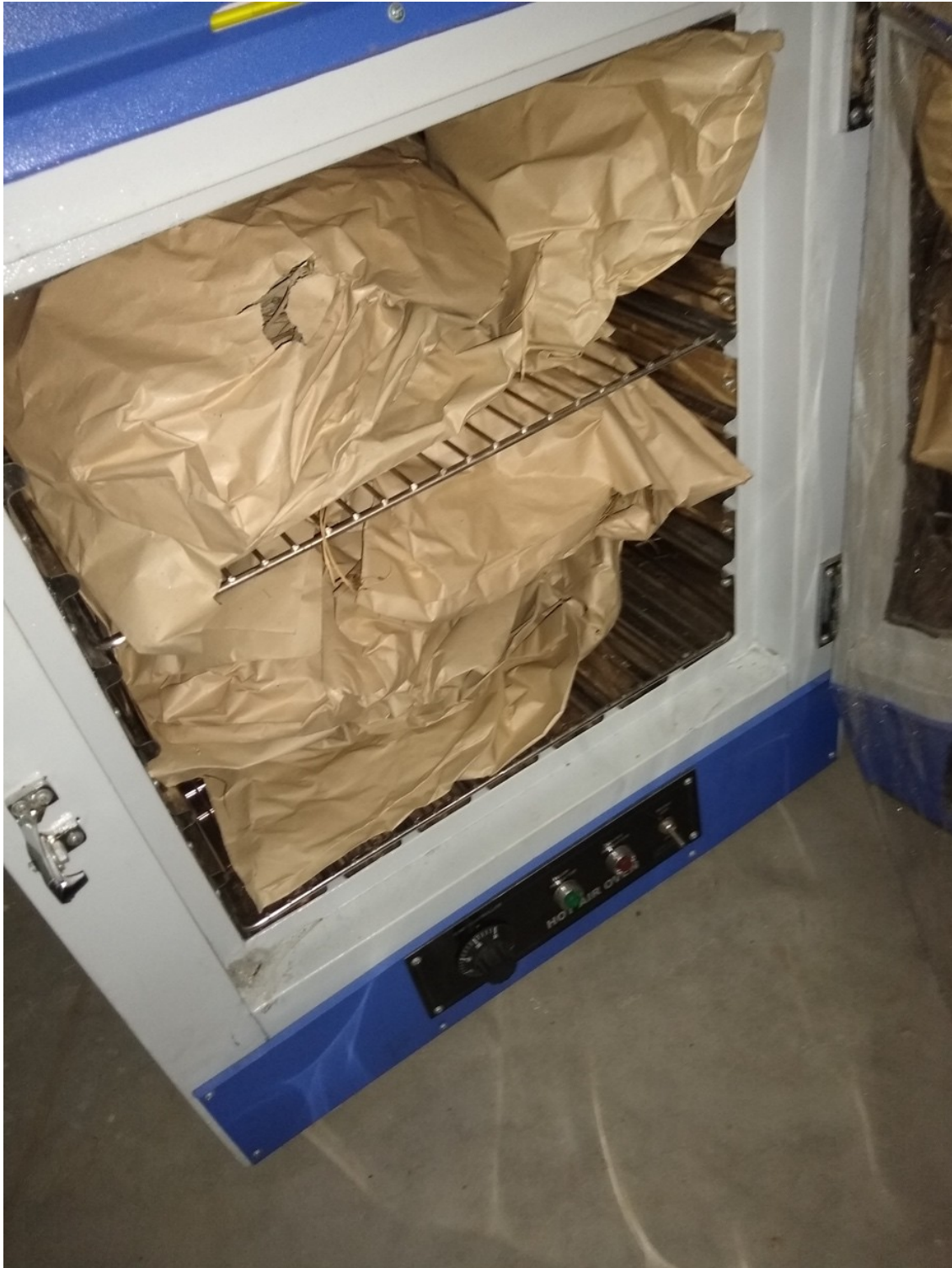
Figure 7: Measuring dried above ground biomass using hot air oven. The enclosed plant material is heated for 6 hours at 80 degrees, and then weighed.
